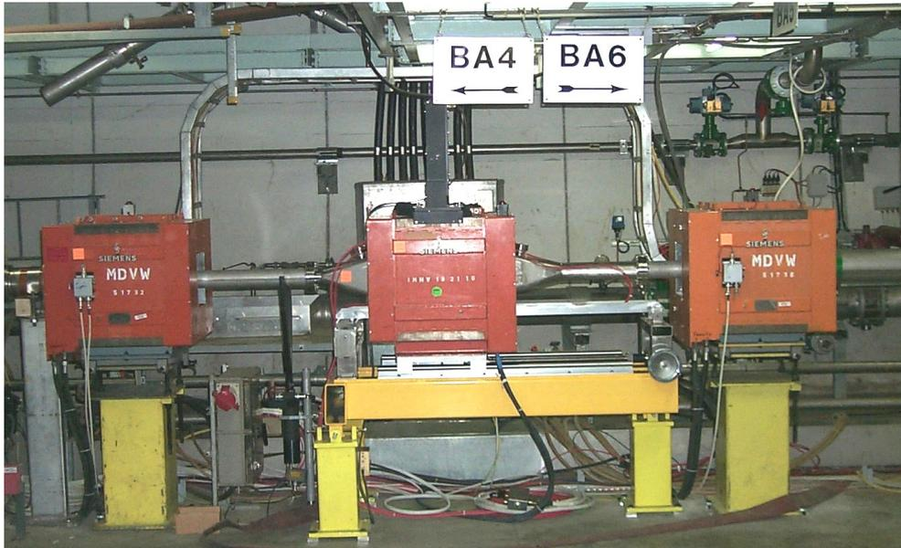
Figure 1.3: *One of the IPMs location in the SPS tunnel. The IPM is situated inside the centre orange magnet. Photo courtesy of J. Koopman [1].*
