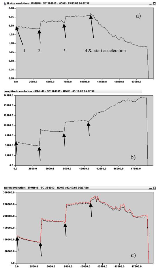
Figure 4: Evolution of: a) the horizontal beam rms, b) the amplitude and c) the integral of the IPM signal during injection then acceleration of 4 batches of 72 bunches of  $1.1 \cdot 10^{11}$  protons.
