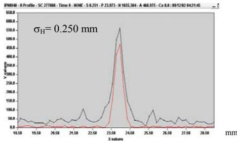
Figure 2: Profile of a bunch of  $5 \cdot 10^{10}$  protons.
